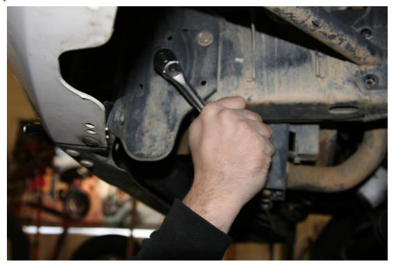
F. With the bumper lose and rotated forward and down a little use a 12mm ratcheting wrench to remove the two bolts per side holding the bumper support to the top of the bumper.
