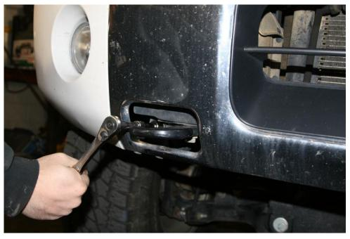
E. Using a 17mm socket remove the two bolts holding the bumper brackets to the outside of the frame on each side.
