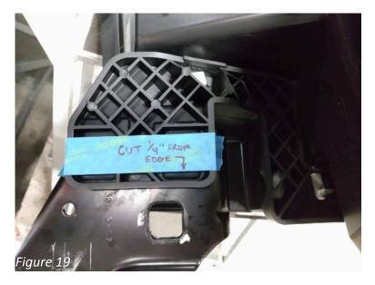
23.\* Using a small reciprocating saw, trim the lower louver shroud as shown. (Figure 20-22)
