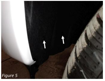
5. Starting on one side of the vehicle, pull outward on the valence to release the clips which attach it.
