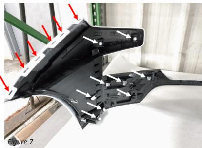
6. Now the grille can be removed by pulling outward on the pieces over the headlights which have two (2) clips first then on the center which has three (3) clips. (Figure 8)
