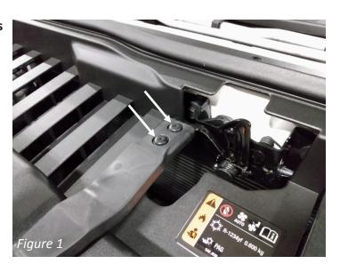
2. Using a panel pry tool, remove the nine (9) push pins in the under-hood cowl to remove it. (Figure 2)
