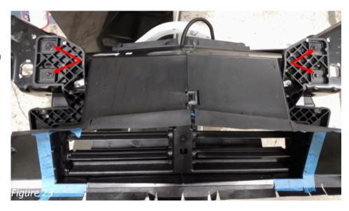
25.\* Reinstall the previously removed lower louver set onto the vehicle by reinstalling the four (4) previously removed push pins from the top of the louver shroud and reconnect the electrical harness. (Figure 24)
