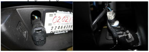
2. Carefully remove the plastic cover on the top of the bumper using your hands only. Start at one end and work each clip slowly to prevent damage to stock components.
