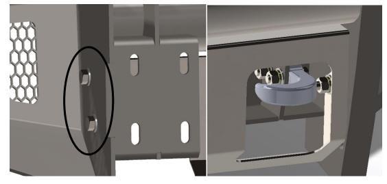
Figure 10a (bolt location for lower guard)
