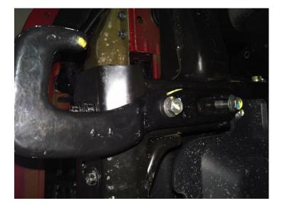
7. Remove the bumper mount brackets from both frame rails using a <u>14mm socket</u>. Save this hardware for later use.
