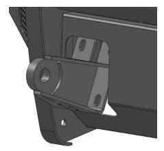
4. **OPTIONAL**: If installing the 2" receiver hitch accessory, attach it to the bumper with the provided ½" hardware
