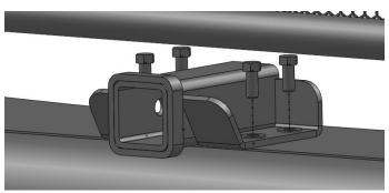
Figure 2 - Hitch Installation
