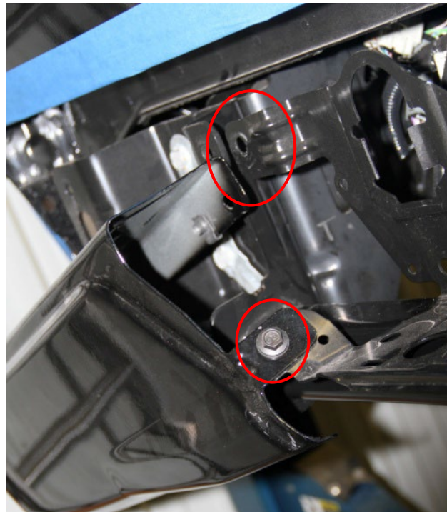
Figure 3b (2x per side, Inner bolt locations)
